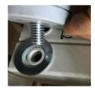
Fit large washer over Rivnut on underside of post horizontal, then tighten castor bolt using an 18mm Gooseneck ring spanner.
