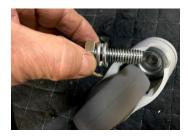
Fit 2 spring washers onto bolt and put into the inside of the castor
