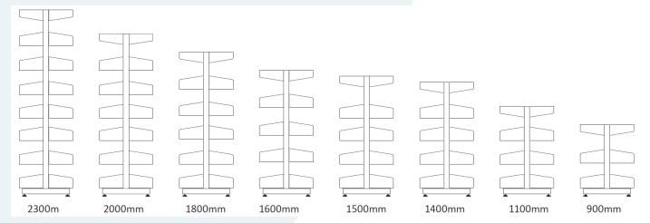
900, 1100, 1400, 1500 & 1600mmH bays can be made as mobile bays this will increase the overall height of the shelving by 140mm
